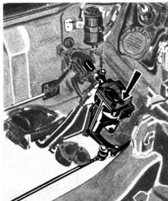
The ball and socket joints of the rods **do not require any lubrication**. The turning circle may be adjusted by means of the screws indicated in the diagram.
