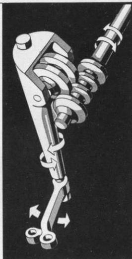
The ball and socket joints of the rods do not require any lubrication.
