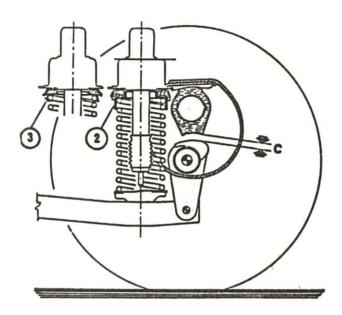
Note - To adjust, remove the seat 3 and add shims in 2 as shown.
