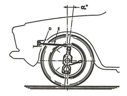
N.B. - Before checking the caster angle shake the front end of car in order to allow the rubber bushing on the front slanting arm to set properly.
