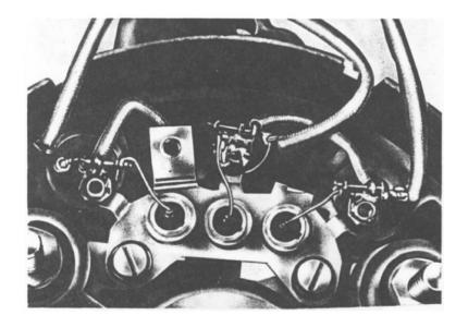
After the field diode bracket has been fitted, connect by soldering the stator, negative diode and field diode leads. When soldering, great care should be taken to avoid overheating the diodes.
