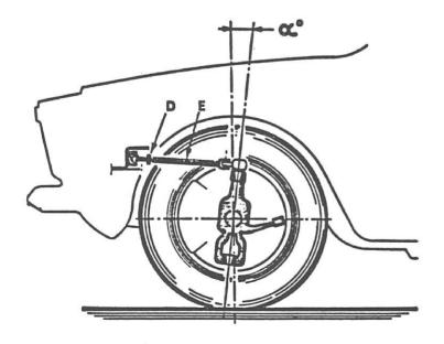
The difference in caster angle between R.H. and L.H. wheel must not exceed 0° 201.
