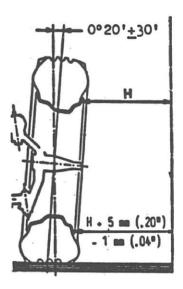
Note - Not adjustable. Check the chassis and suspension arms if necessary.
