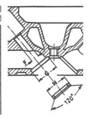
Interference between valve seat insert and recess in cylinder head . . . H-G .100 to .040 mm (.0039 to .0010")
