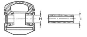
End play of the connecting rods on the crankpins G .200 to .300 mm (.0079 to .0118\*)
